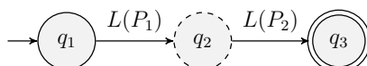
Figure 2.7: Thompson sub-automaton for concatenation. This figure shows the Thompson sub-automaton for concatenation: an internal node corresponding to P_1 \cdot P_2 , for sub-patterns P_1 and P_2 . This automaton will accept the family of strings \{xy \mid x \in L(P_1) \text{ and } y \in L(P_2)\} . The dashed node q_2 represents the former accept state(s) of the sub-automaton for P_1 , which may no longer be the accept state(s) of the combined sub-automaton for P_1 \cdot P_2 .
