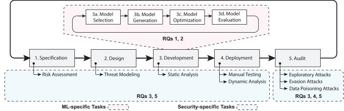
Figure 1: An engineering lifecycle for machine learning-based IoT devices. It combines several models including the SDLC [2, 28, 53].
